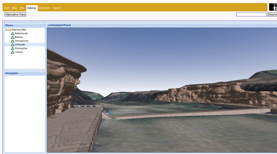
Figure 4: 3D surface Model of stone walls with caves derived from terrestrial laser scanning in the Valley of Wofoyuan
